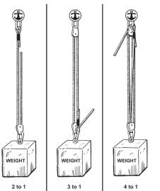
Build your mechanical advantage systems with care for angles, load directions and load limits.
